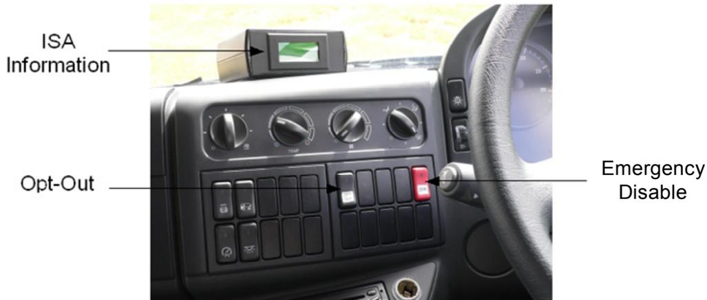
**Figure 29: HMI in the ISA truck**
