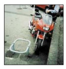
The UK photograph above shows one of the many different possible forms of solid security point in a motorcycle parking area. Others include better protection for pedestrians with a waist high slatted fence erected at the loop to ensure that it does not present a hazard.
