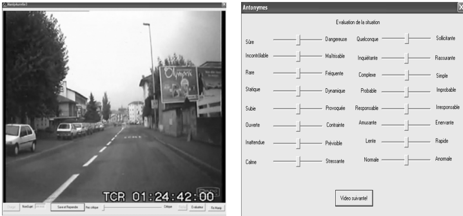
Fig.1. Synthetic view of the Risk Awareness Measurement Tool, including a Likert Scale (on the left, below the road scene view) and an Osgood Semantic Differential (on the right)
