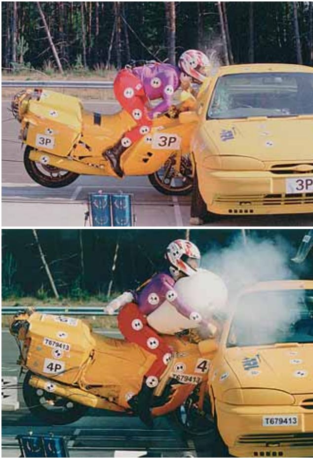
Figure 12 Impact at 90° without and with the TRL/Lotus Engineering airbag system
