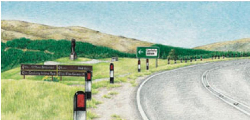
In this option the side road ahead warning sign has been removed. The large advanced direction sign has been reduced in size, lowering it to below the skyline. The tourist sign has also been lowered to prevent it obscuring the monument. However, the verge marker posts, the verge and the tourist sign continue to present an intrusive image.
