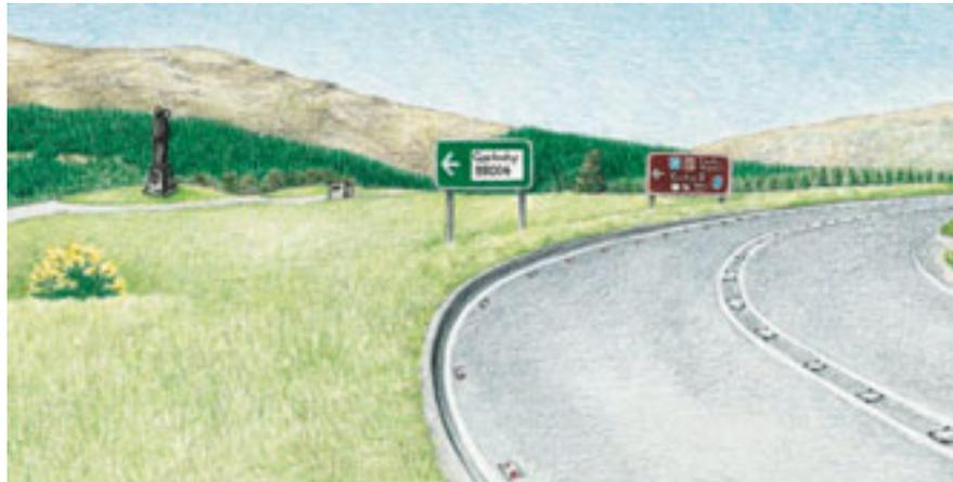
This final option offers a further simplification by placing both signs on a single structure. This increases the height and breaks the skyline but presents a lower impact overall.
