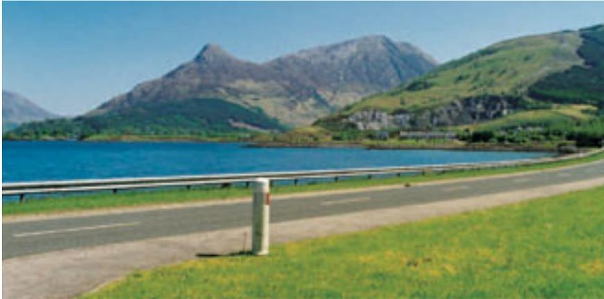
This shows a very long length of continuous safety fencing which, while necessary, also has a visual impact on the scene beyond. The impact could be reduced by painting the fence a duller, more neutral colour.
