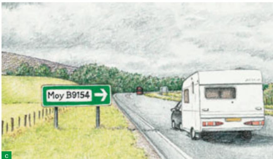
c A further option reduces both the height and size of the sign, while providing adequate information. The safety fence can also be removed since the diameter of the posts has been reduced.
