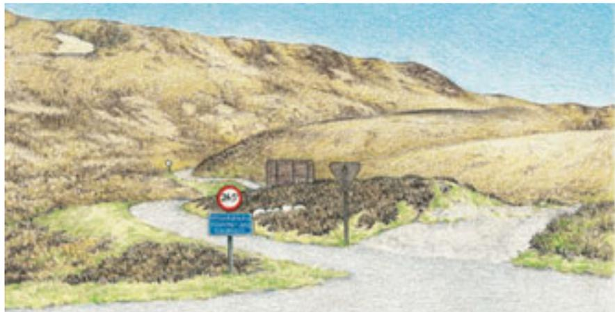
In this option the impact has been reduced further by combining the 'give way' and weight limit signs into one double-sided structure.
