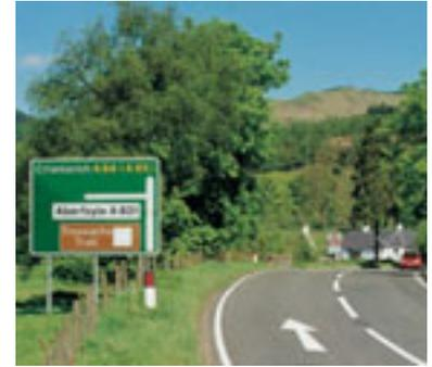
Although this is quite a large sign for the scale of the landscape, it has been set against a backdrop of trees which helps to tie it into the scene and keeps its impact to a minimum.
