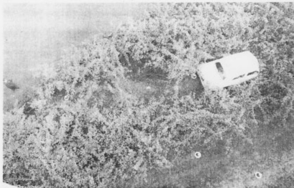
Overhead view showing final position of test car in hedge of rosa multiflora Japonica
