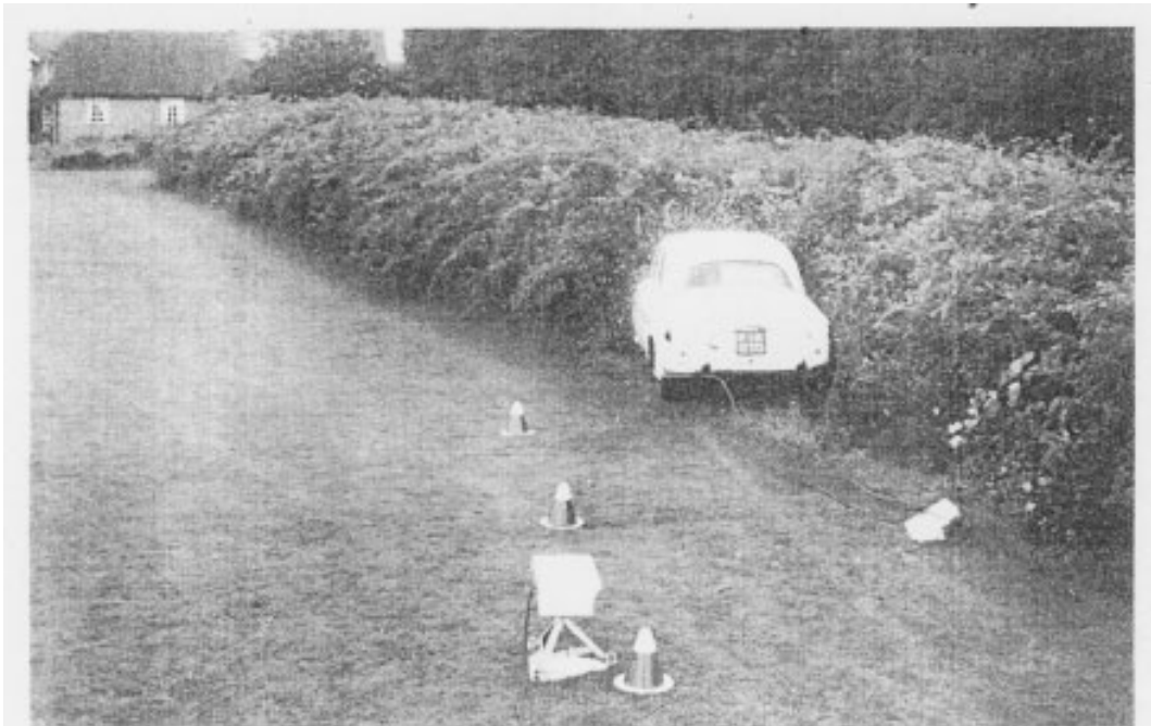
Test car at start of impact with hedge of rosa multiflora Japonica
