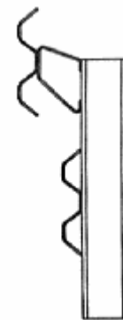
Fig. 3: Fitting of an additional W beam
