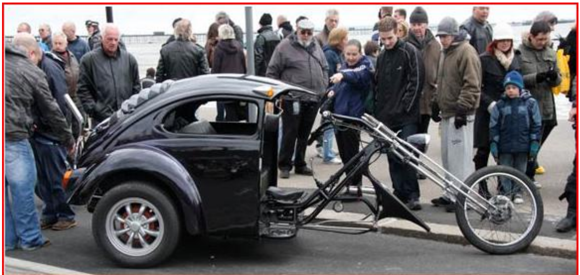
Hybrid Trike with motorcycle front end and Volkswagen Beetle rear end
